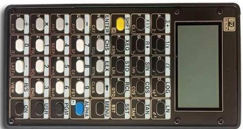
The **PX-41CX** programmable calculator is a calculator that incorporates the functionalities and language of the HP-41CX calculator thanks to an emulation running on an AVR128DA microcontroller.
